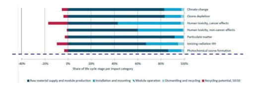
Life cycle analyzes carried out for PV installations highlight the potential for more sustainable PV production and installation. The graph clearly shows that the greatest potential for all Product Environmental Footprint Category (PEFCs) lies in material flow and production towards the module (see also: <a href="http://www.etip-pv.eu/fileadmin/Documents/ETIP">http://www.etip-pv.eu/fileadmin/Documents/ETIP</a> PV Publications 2017-2018/181122 - ETIP PV Report on PV Quality and Economy web.pdf)
