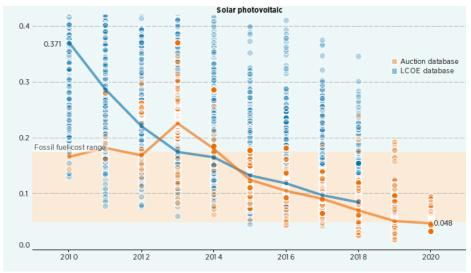
Levelized Costs of Electricity (LCOE) in US\$/kWh for solar PV projects. Source: Future of Solar Photovoltaics, Report, IRENA, 2019
