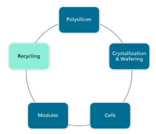
At the end of the life cycle nearly 100 % of the parts of a module will be made available for a new life cycle. The cost for the recycling process must be considered at the beginning of the cycles.
